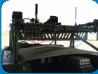
Omni antennas on light vehicles for army patrols
